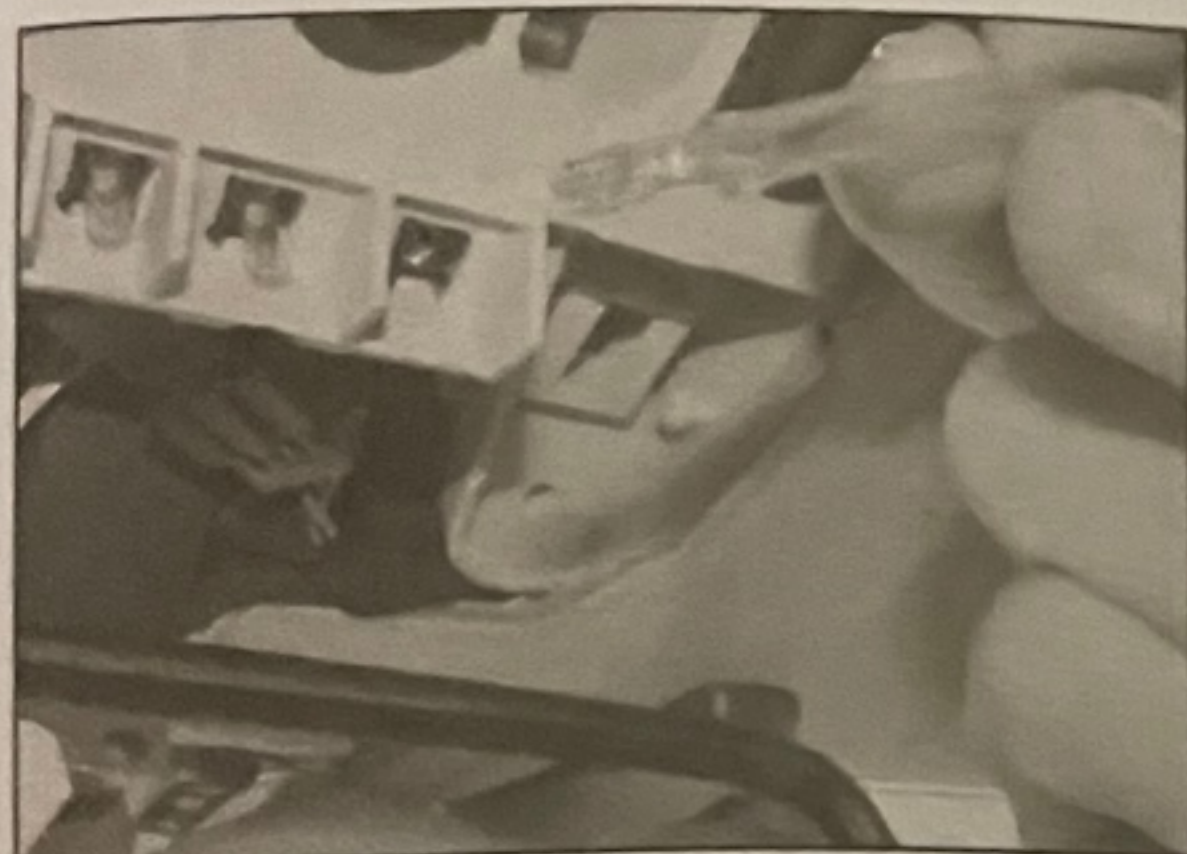
5.24d . . . the wedge-type illumination bulbs
