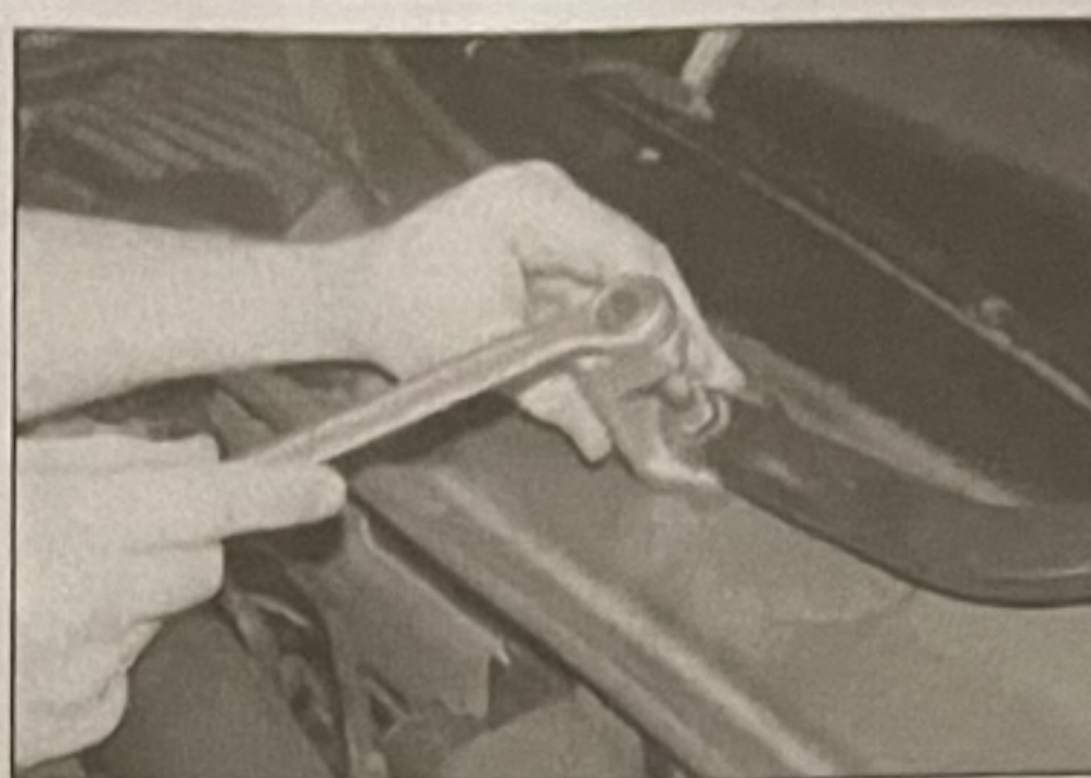
13.4 . . . then use a small puller to remove the wiper arm from the spindle
