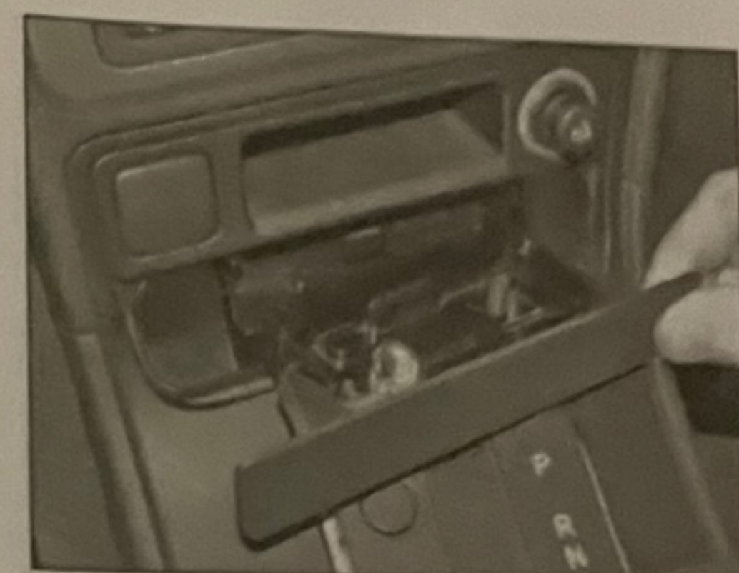
5.27 Removing the outer trim panel from the ashtray
