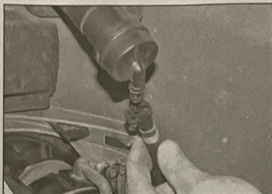
16.5b ... disconnect the washer pipe...
