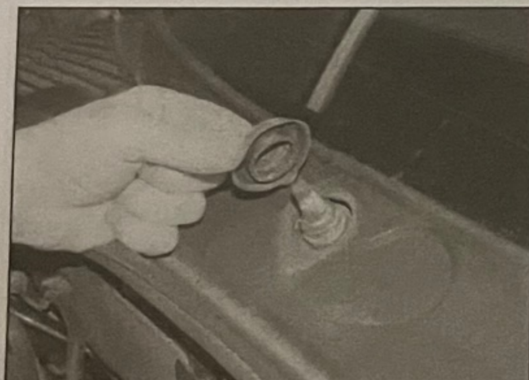
15.2 Removing the rubber seals from the spindles
