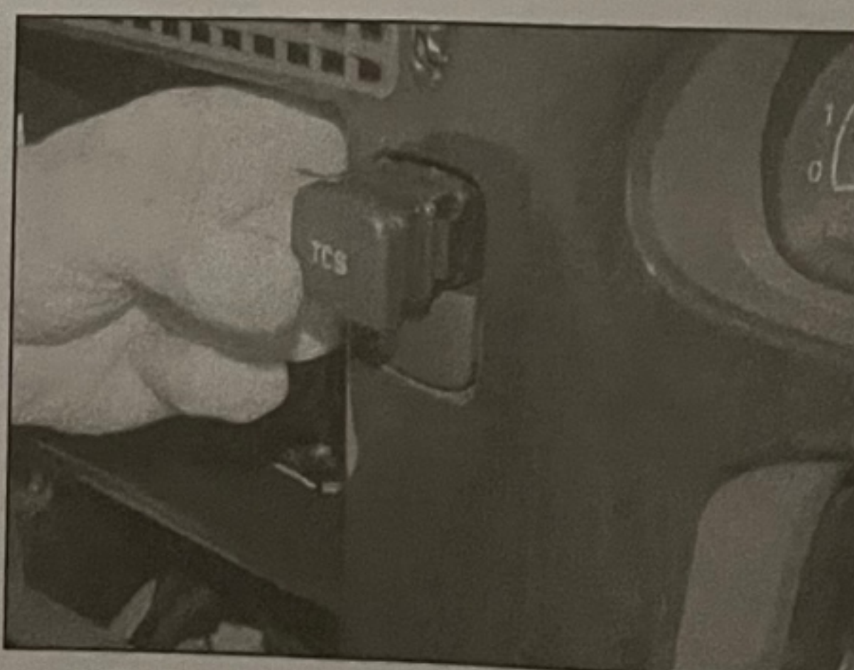
4.39 Removing the TCS switch (early models)
