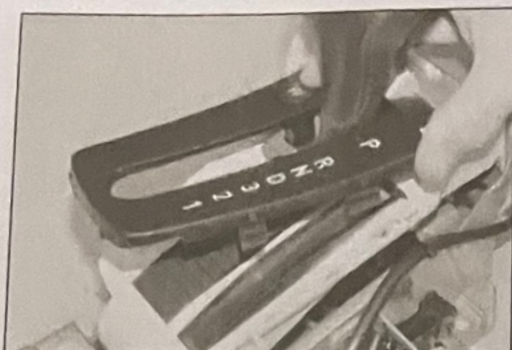
5.35a Remove the position indicator panel...
