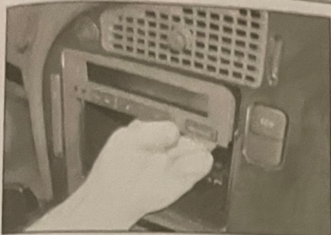
10.3a Reach through the radio/CD player aperture and push out the SID unit
