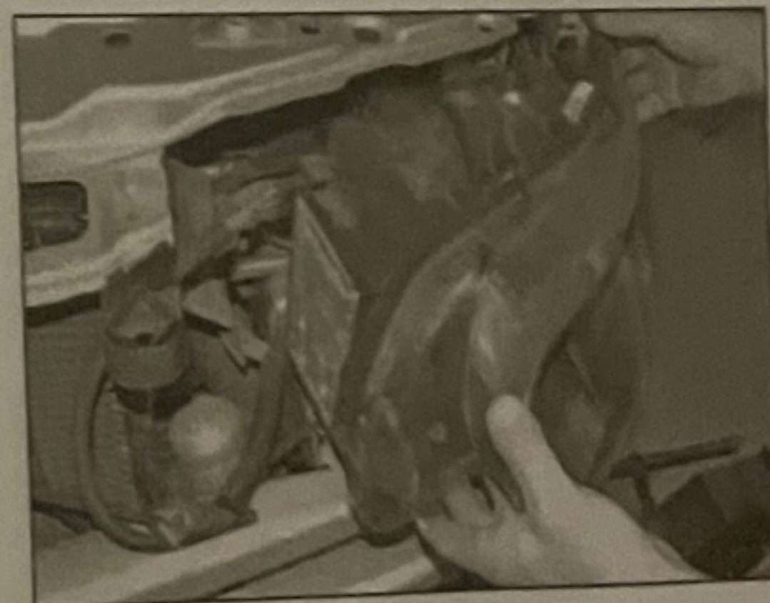
7.3 Withdraw the headlight...
