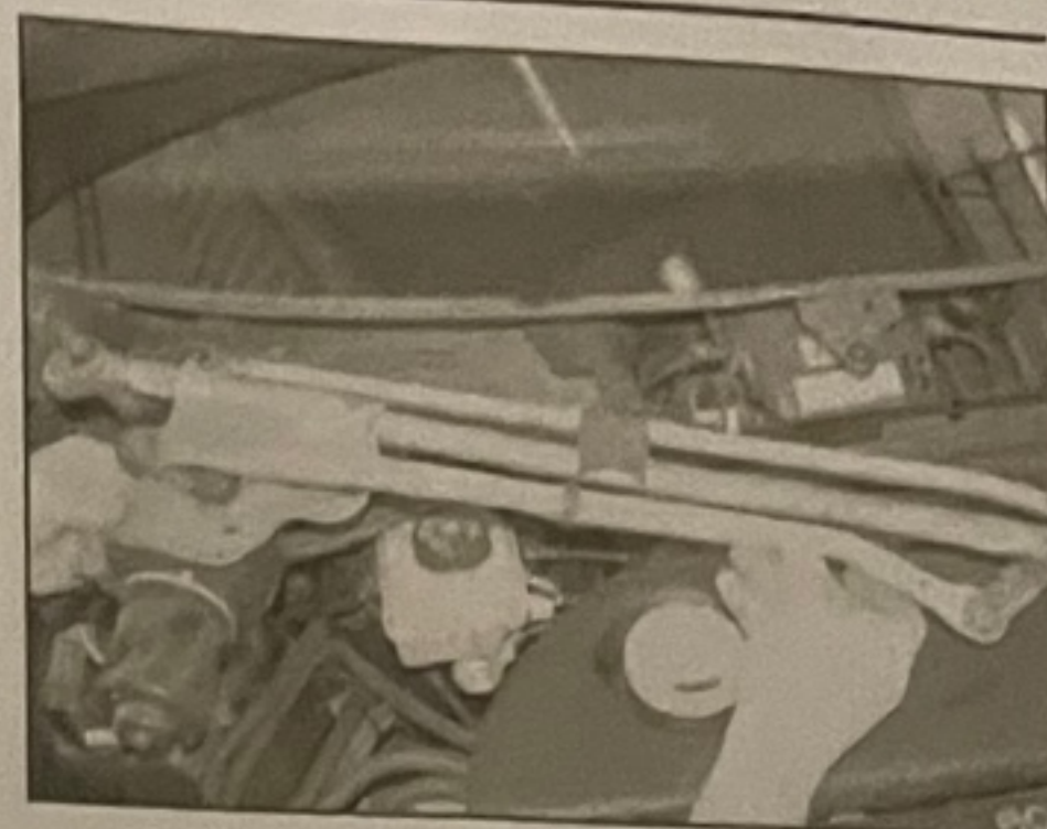
15.6 Removing the wiper motor and linkage
