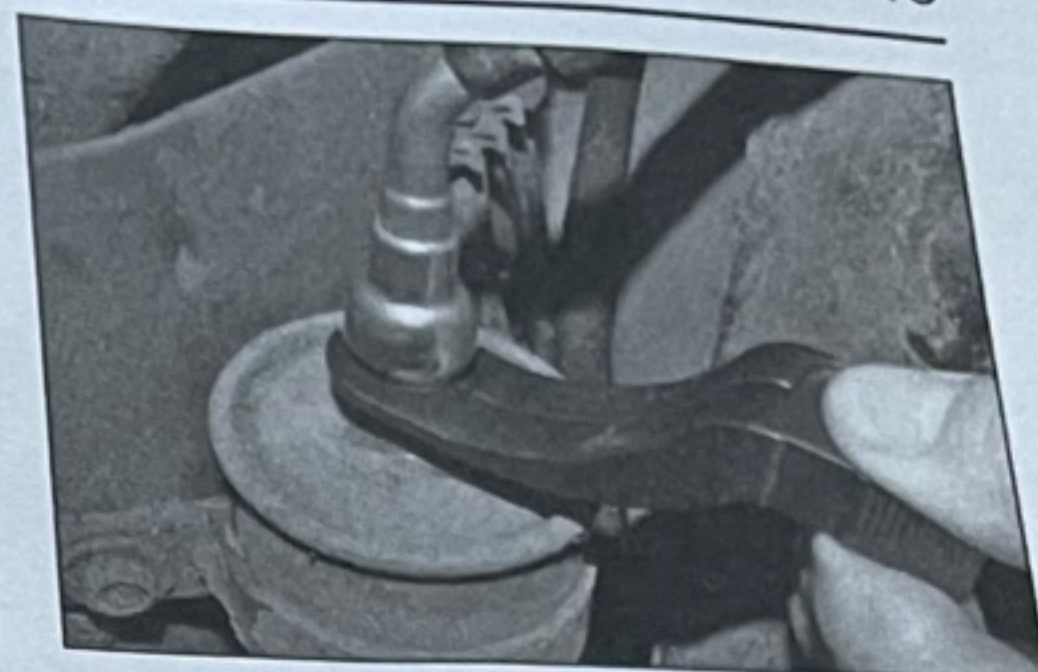
26.7b ... pull the tool into the fuel hose connection ...
