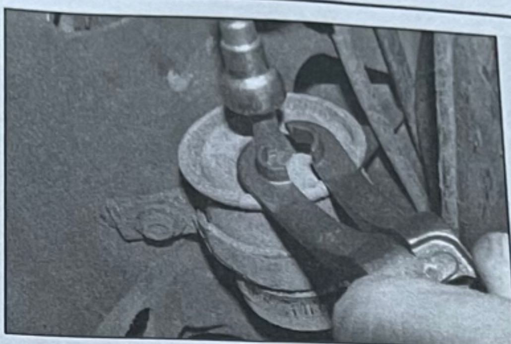
26.7a Fit special tool around filter outlet pipe ...
