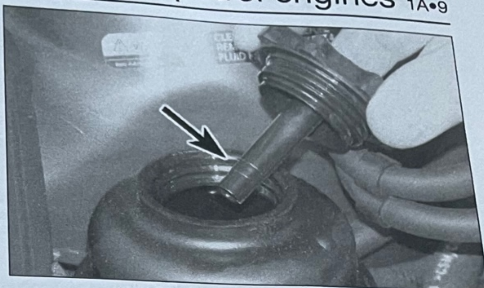
11.3 Fluid level marks on the dipstick
