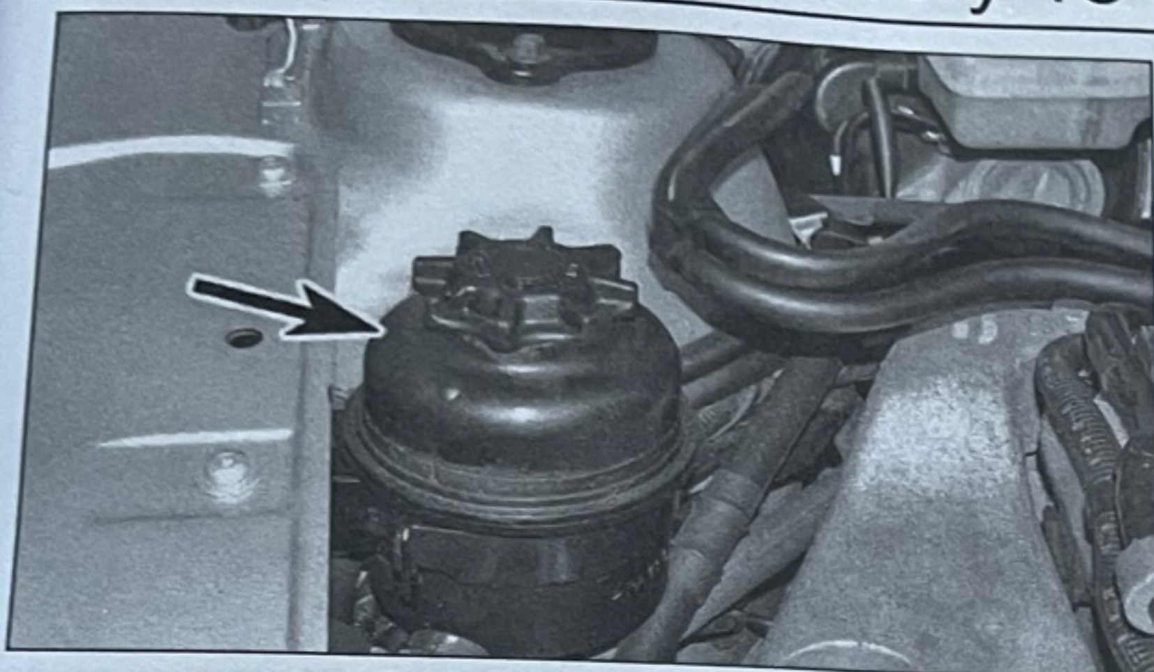
11.1 Power steering fluid reservoir
