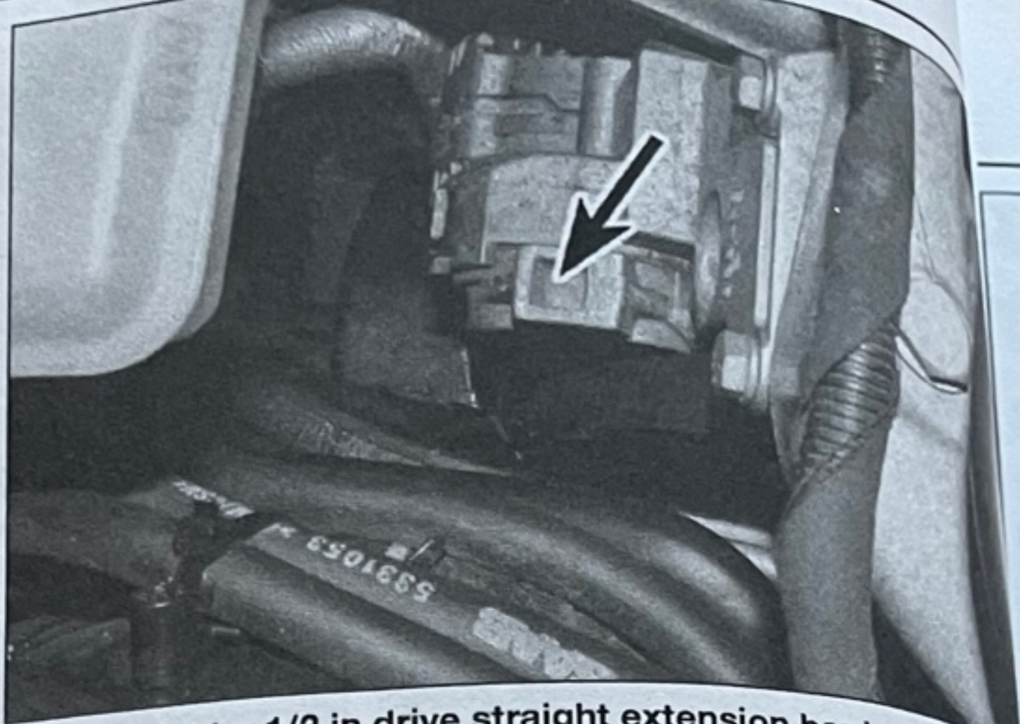
27.3a Insert a 1/2 in drive straight extension bar into lug at top of outboard (moving) part of tensioner ...
