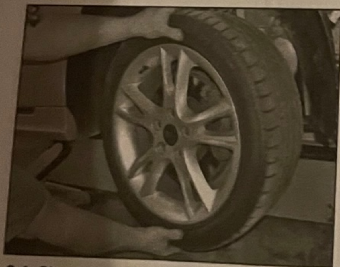
6.4 Check for wear in the hub bearings by grasping the wheel and trying to rock it
