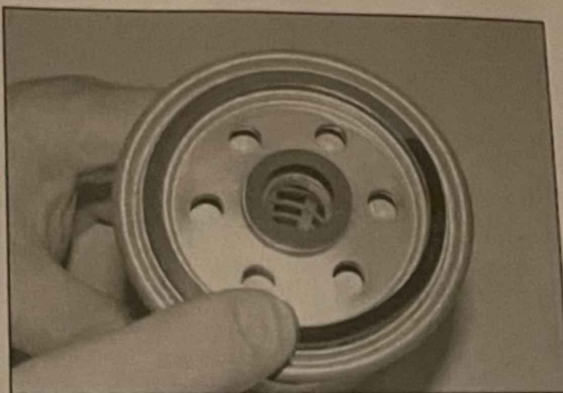
22.5a Lubricate the filter seal with clean fuel ...
