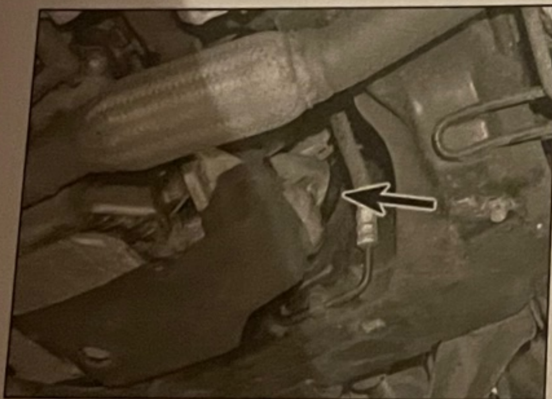
3.8a Unscrew the housing cap (arrowed) a few turns with a 32 mm socket . . .
