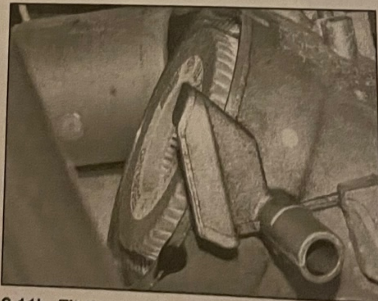
3.11b Fit the new filter into the housing . . .
