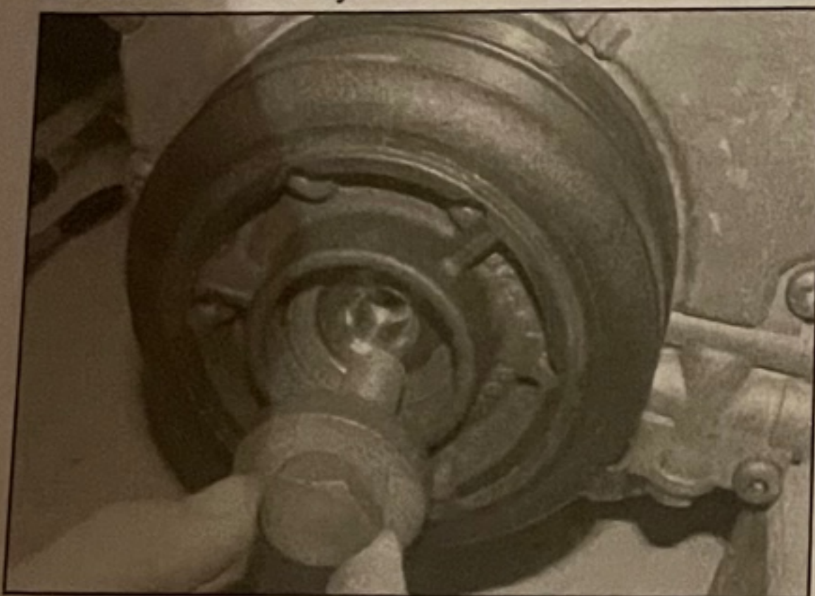
8.6 Remove the crankshaft pulley bolt and withdraw the crankshaft pulley
