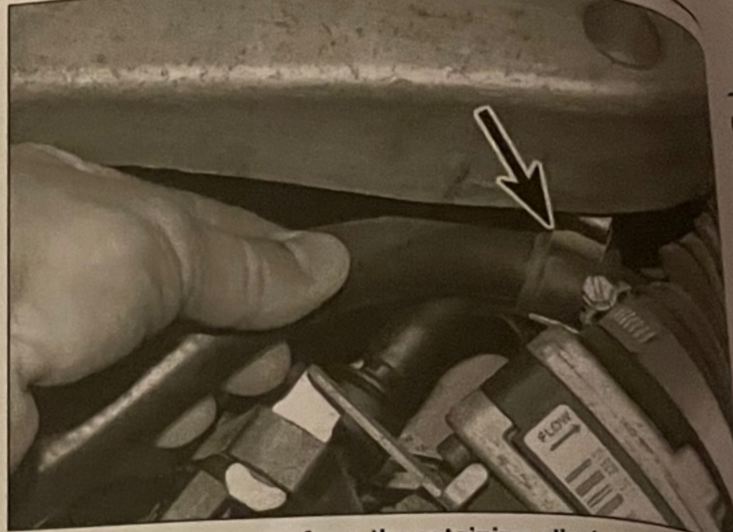
13.11 Unclip the hose from the retaining clip (arrowed) under engine mounting
