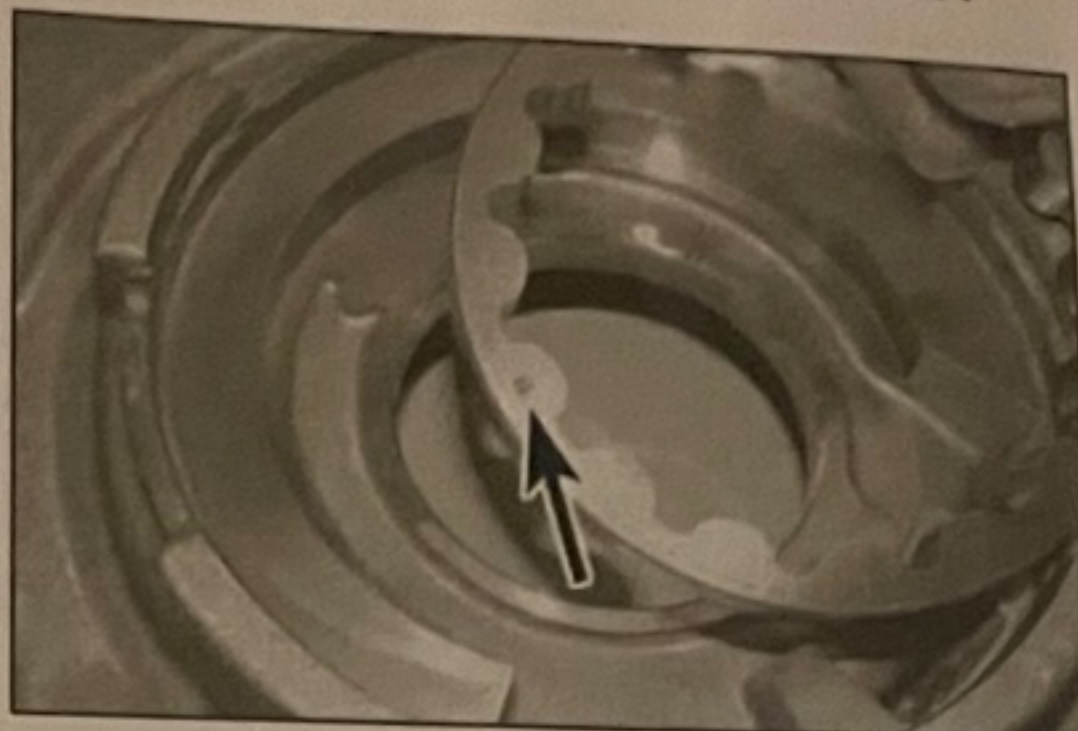
8.11b ... and outer rotor from the timing cover. Note that the position mark (arrowed) is facing outwards
