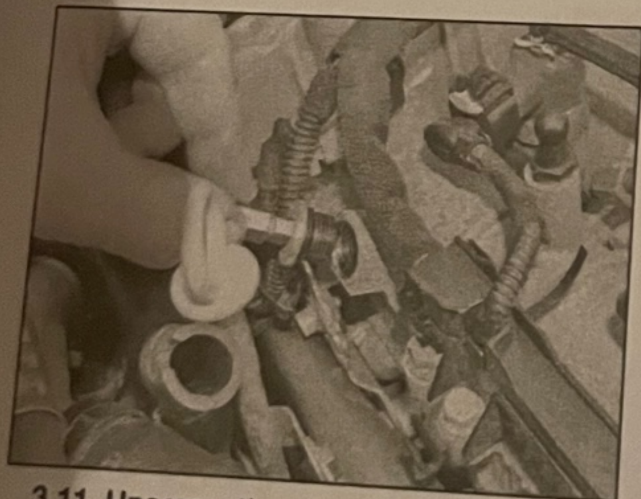
3.11 Unscrew the closure bolt from the valve timing checking hole in the camshaft housing
