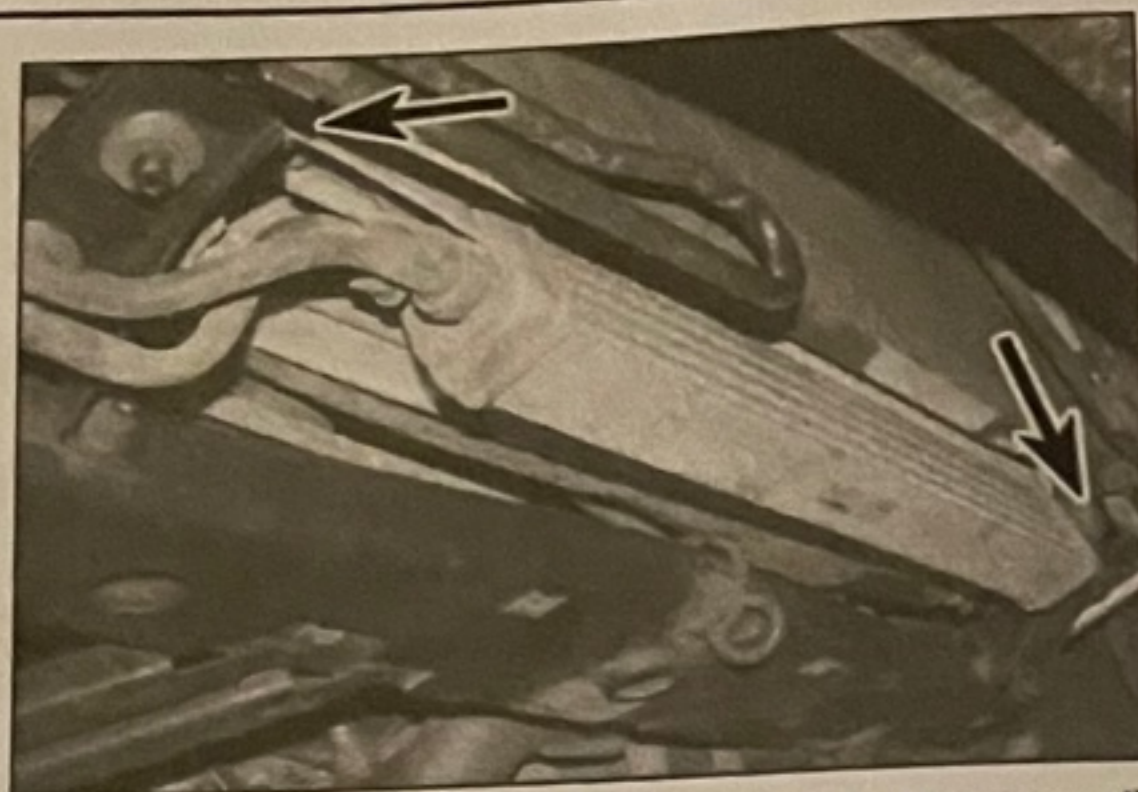
4.28b . . . and the retaining bolts (arrowed)
