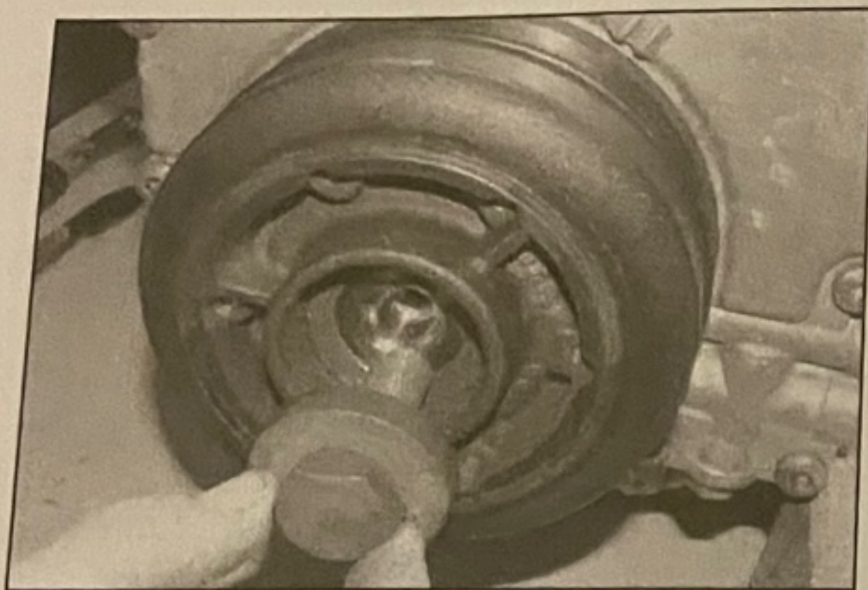
9.6a Remove the crankshaft pulley bolt ...
