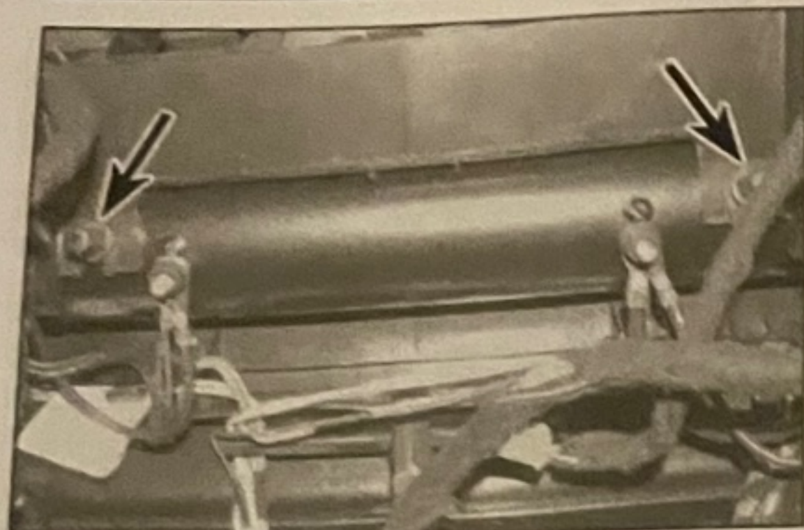
9.23 Nuts securing the wiring loom support to the crossmember
