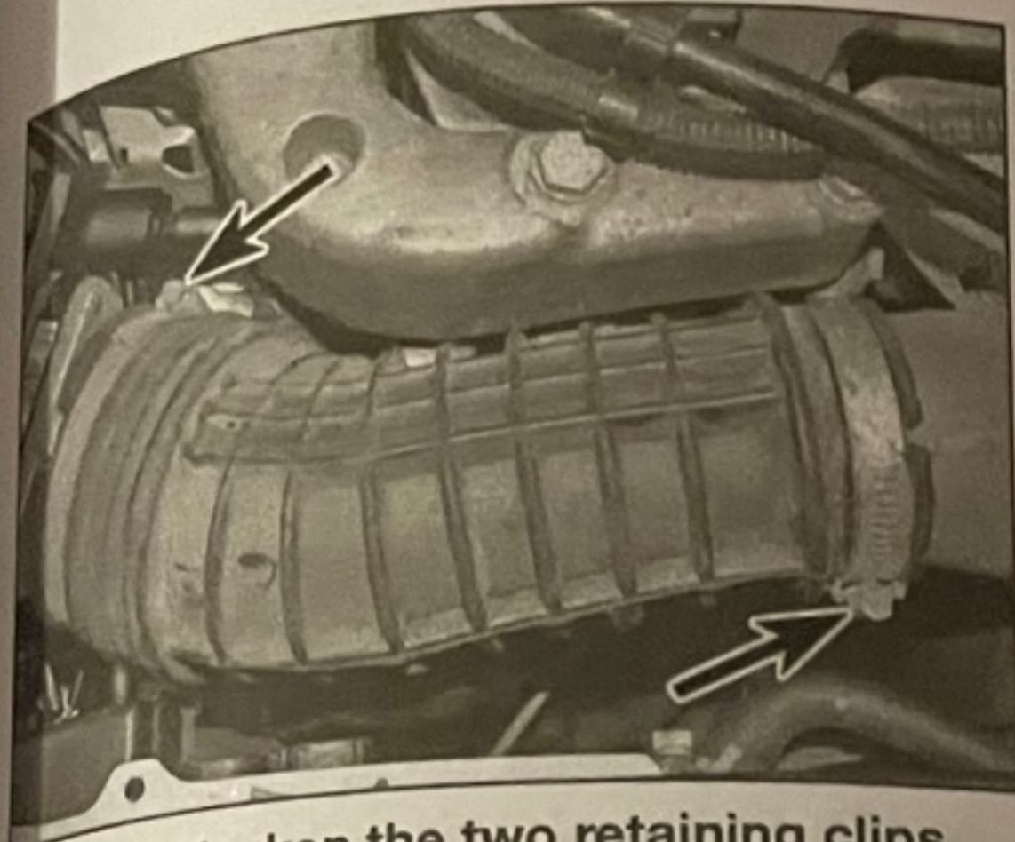
14.13 Slacken the two retaining clips (arrowed)
