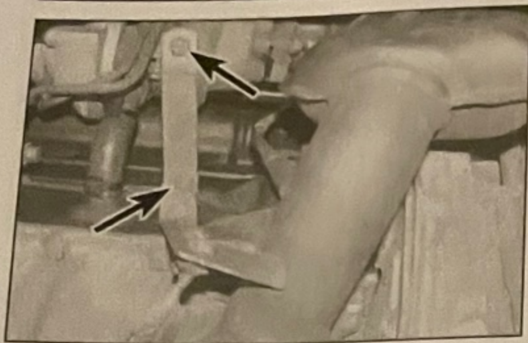
16.3 Undo the two retaining bolts (arrowed) from the exhaust stay bracket
