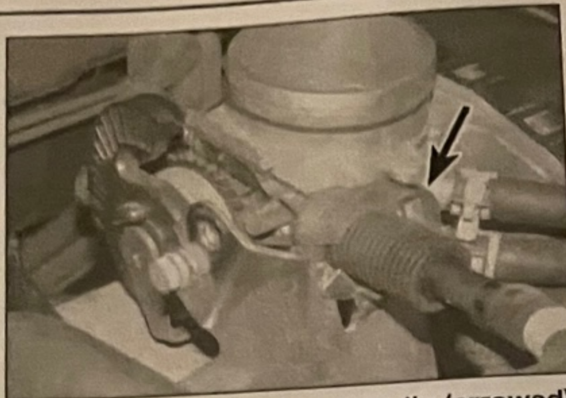
3.6 Remove the outer cable clip (arrowed) securing the accelerator cable to the bracket
