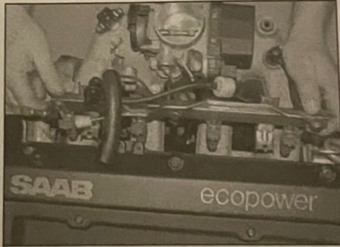
14.48b ... then withdraw the fuel rail from the intake manifold
