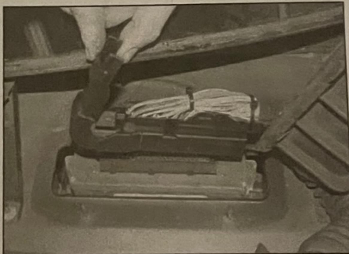
14.4 Unclip the multiplug wiring connector from the control module
