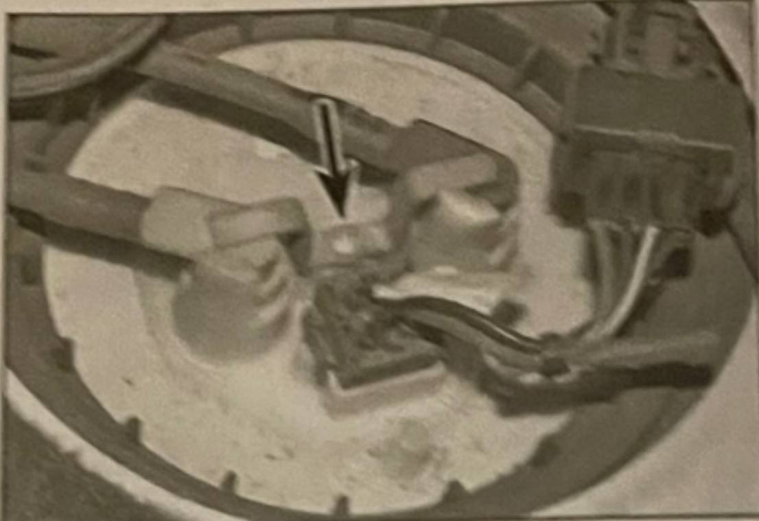
9.4 Undo the retaining screw to release the fuel pipes from the pump
