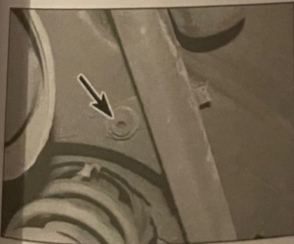
12.7 Undo the fuel filler pipe retaining bolt (arrowed)
