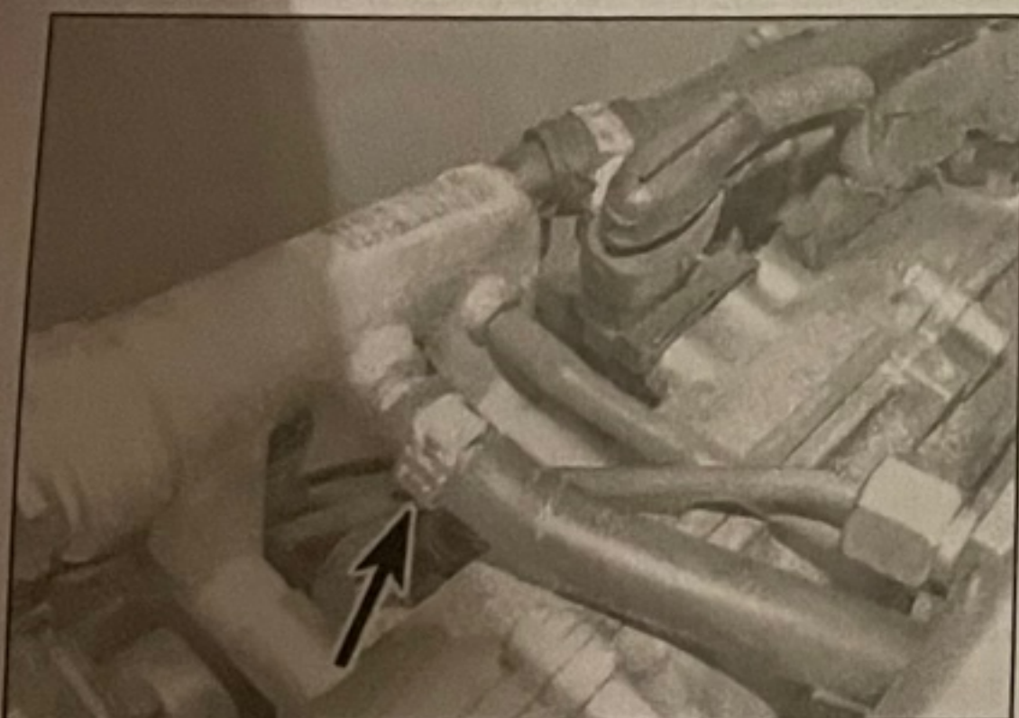
10.4a Release the clips and disconnect the upper (arrowed) . . .
