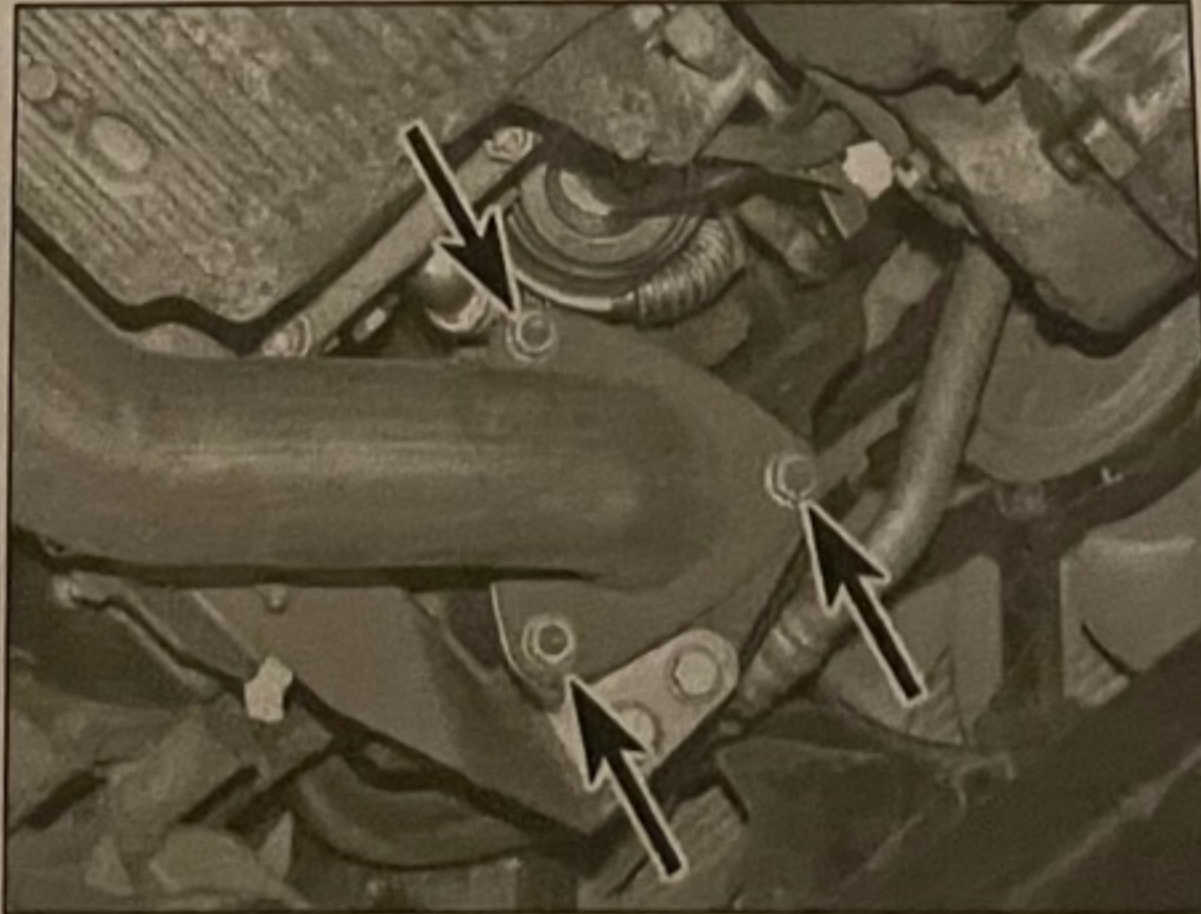
18.7 Undo the 3 nuts (arrowed) and detach the front exhaust pipe from the catalytic converter
