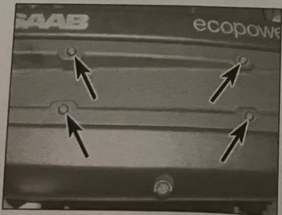
3.2 Slacken and remove the four screws (arrowed) securing the ignition cartridge
