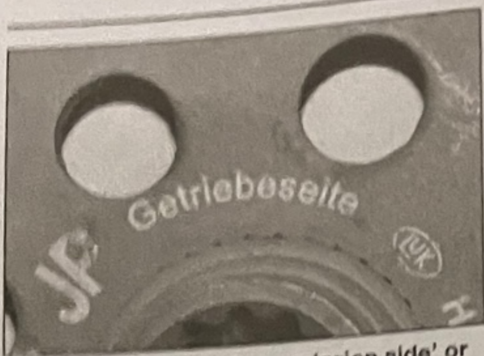
3.20 The lettering 'transmission side' or 'Getriebeseite' on the friction plate must face towards the transmission
