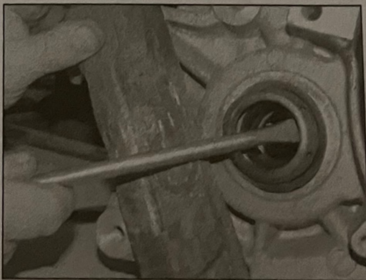
5.5 Levering out the oil seal, using a block of wood to allow better leverage
