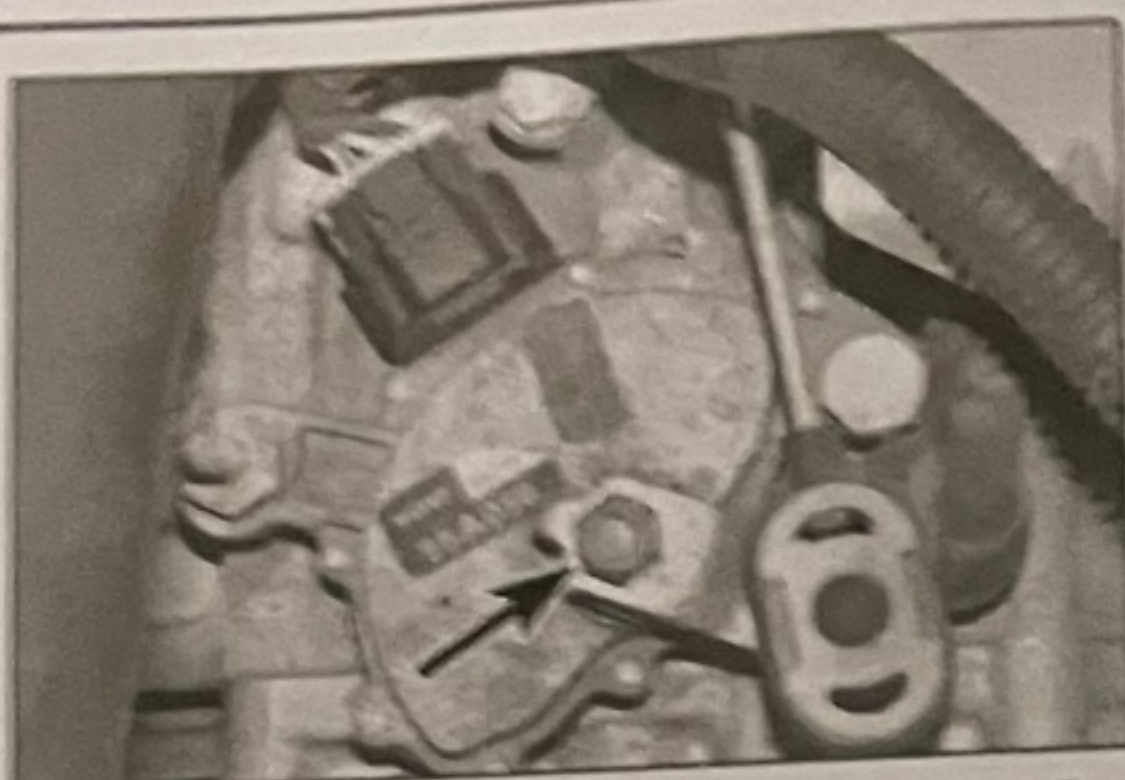
8.5 Remove the retaining nut (arrowed) and detach the selector lever from the position sensor
