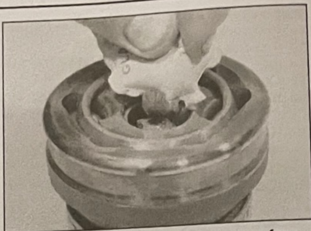
3.13 Pack the CV joint with grease from the service kit
