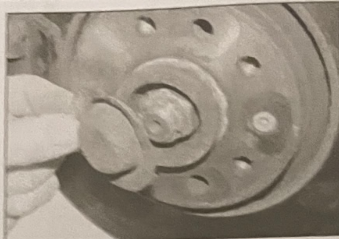
2.2b ... then remove the cover from the hub flange
