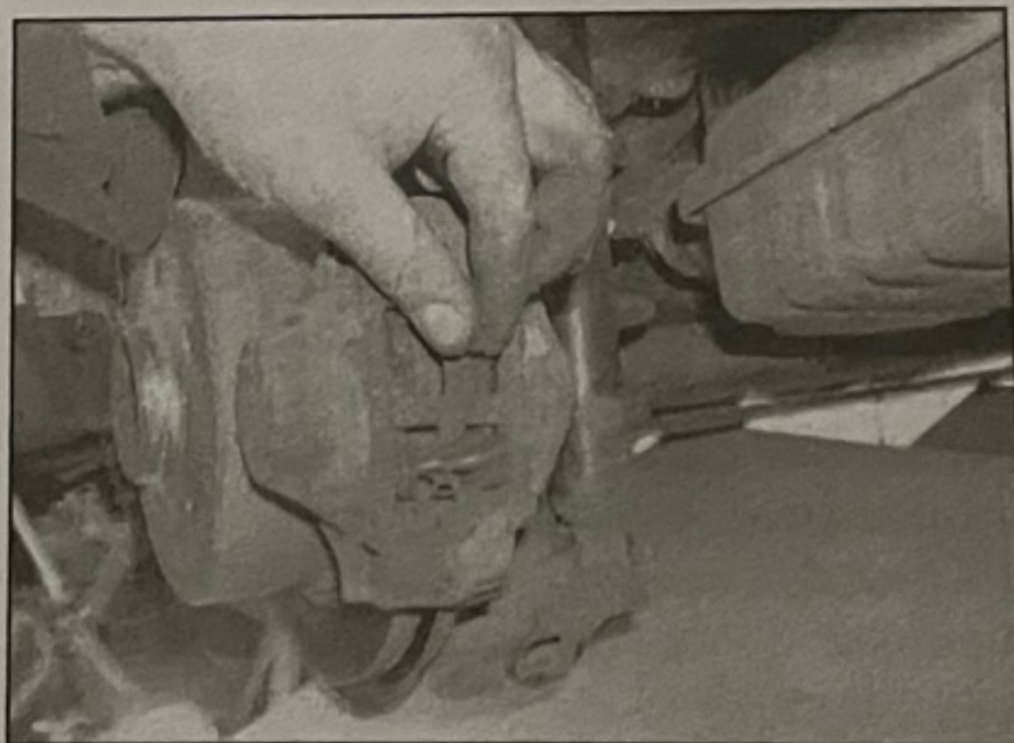
5.3 Removing the anti-squeal spring
