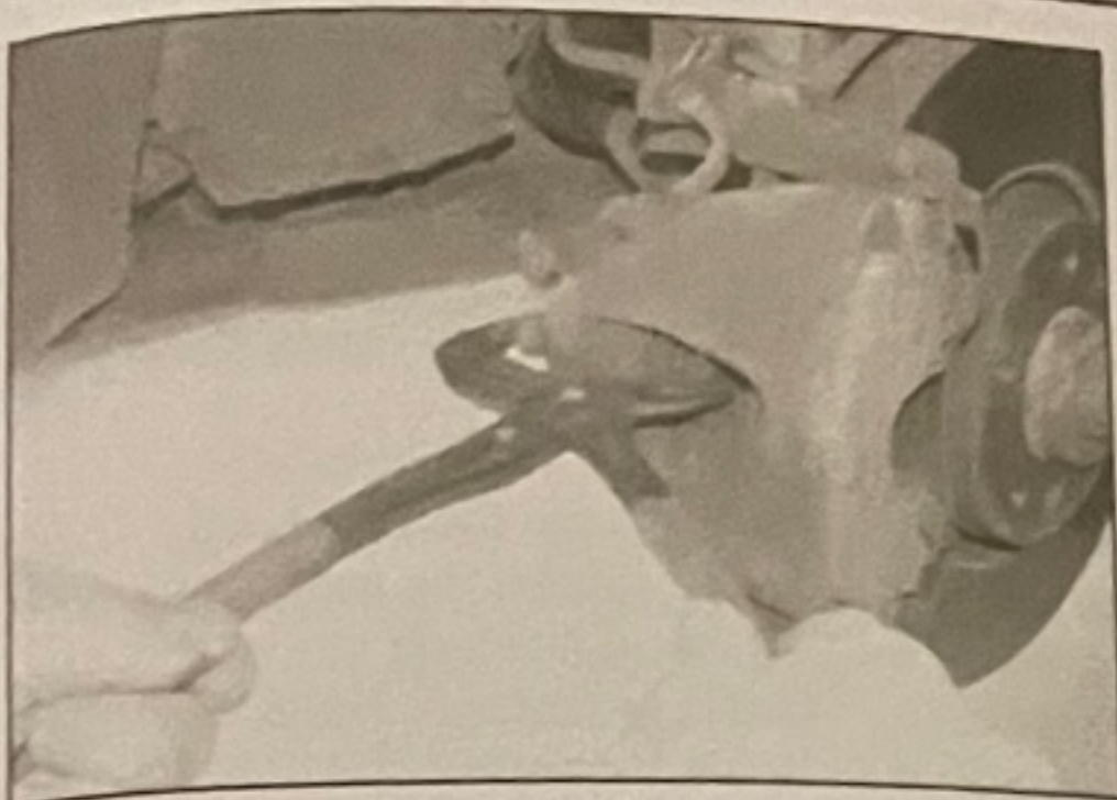
4.2 Using slip-joint pliers to press the piston into the caliper
