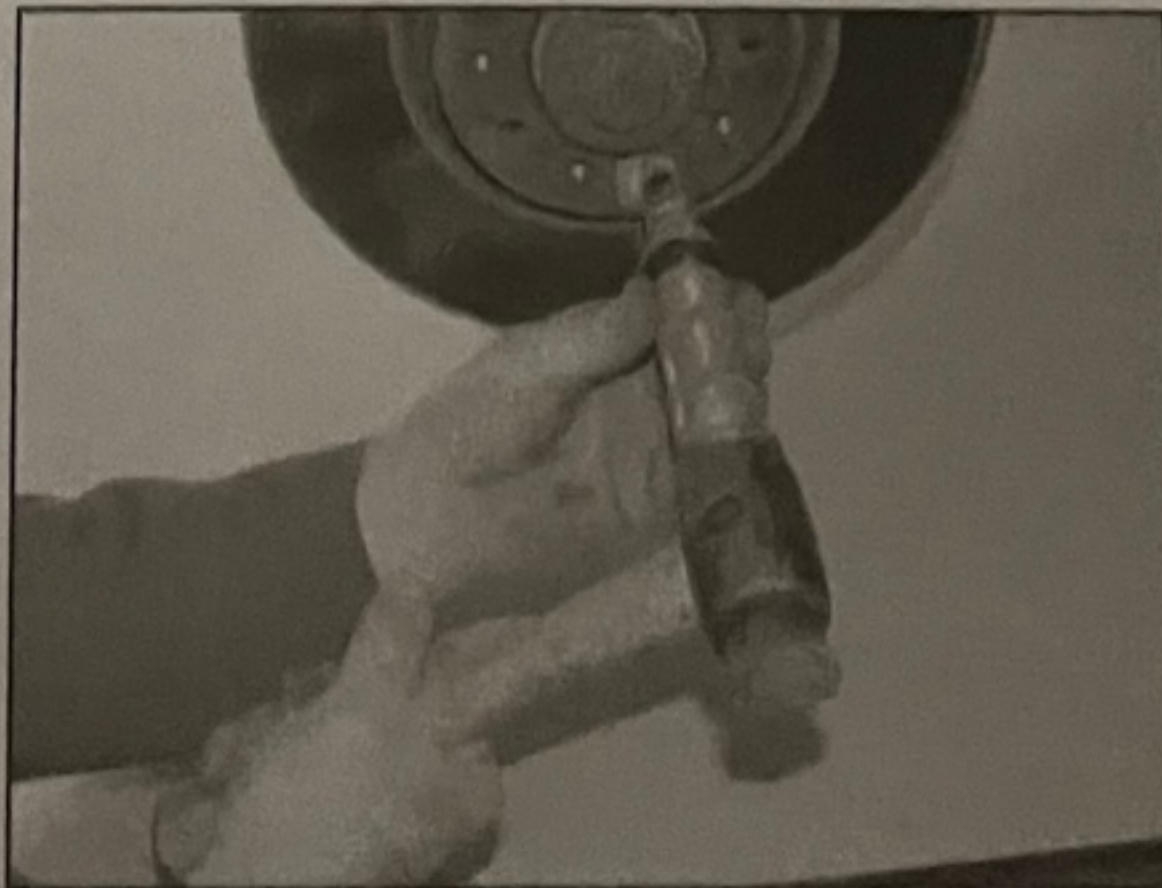
8.11b Using an impact driver to loosen the brake disc securing screw
